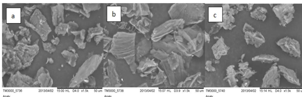
Figure 1. Scanning electron micrographs (x1500 magnification) of passion fruit peel. a) commercial sample, b) freeze-dried sample, c) dried at 60°C sample
